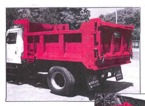
The Air-Flo® Side-Tip body combines a complete exterior body with an inner right side wall joined to an AR-400 floor for unmatched structural support and rigidity. This "body within a body" design allows for superior structural integrity of the body during side tip or rear tip dumping operations.
